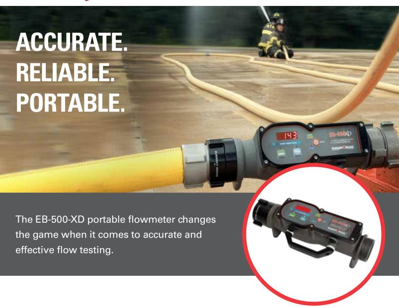
The flow tube, paddlewheel, digital readout, and battery are all self-contained making this unit extremely compact. The waterway features a unique internal waterway shape ensuring laminar flow for consistently accurate readings up to 500 gpm/2000 lpm. The flow pickup is a paddlewheel design which is located further into the middle of the waterway increasing reliability of the flow readings.
